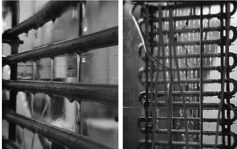
Photo 1. On the left the inter-tube flow showing the jets/jets-droplets type of flow. An oscillating jet falls out of the absorber bundle. On the right the typical spatial wetting transition for the whole absorber is shown.
